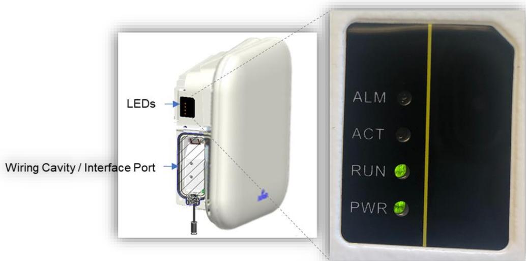
In this figure of the LEDs, the eNB is powered on and running but not yet active and has no alarms.
