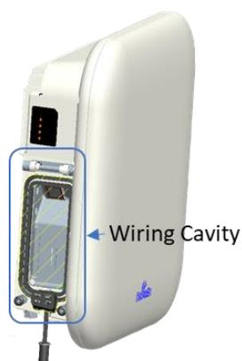
2. Connect the Ethernet cable to the **ETH** interface in the wiring cavity.
